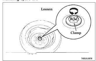
Remove the installation clamp to remove the spare tire. To install the spare tire, tighten the clamp firmly with your fingers until the spare tire has no more play.
